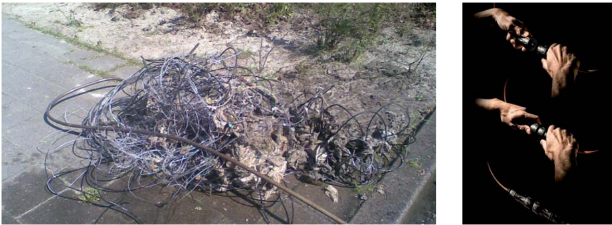
Figure 1. Improper fibre-optic cable handling (left) and newly tested IP68 LC fiber-optic cable connector (right)
